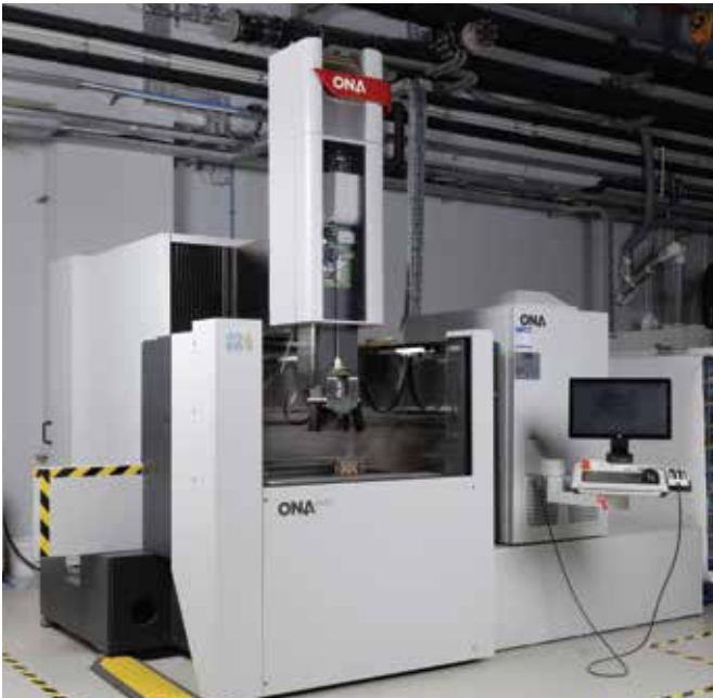
Wire EDM: Dimensions: 1300 x 1040 x 500 mm 3 Wire travel in X-axis: 800 mm, Y-axis: 600 mm, Z-axis: 600 mm Maximum cutting speed: 450 mm 2 /min
