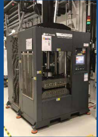
Hot Press: Dimensions : 500mm x 500mm Pressure Force: 50 tons Temperatura: 400°C
