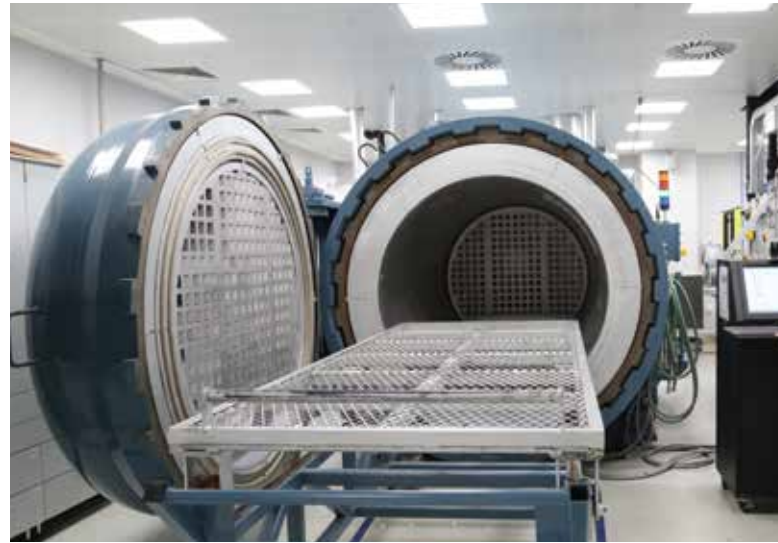
Autoclave; Diameter 1.5Mt , Length 3.0 Mt Pressure 20 bar, Temperature up to 400°C
