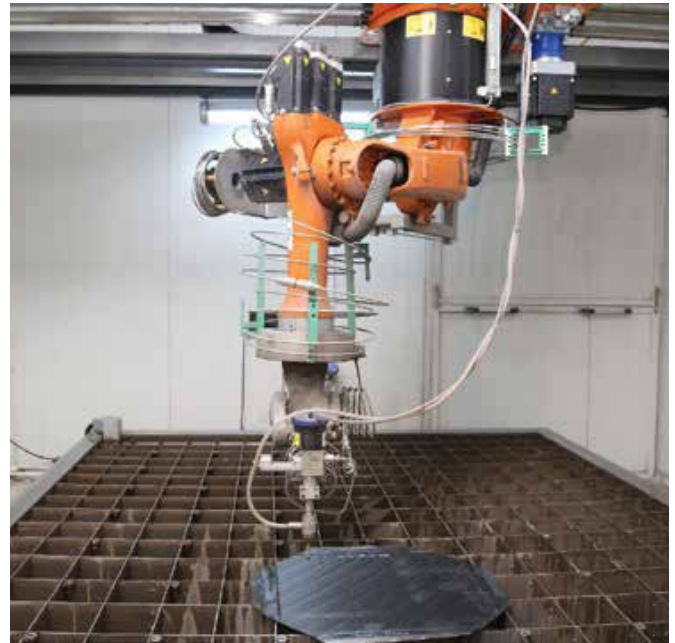
Abrasive Waterjet: Capable of performing 3D cutting Pressure up to 3750 bar
