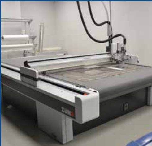
Digital Ply Cutter Working Dimensions: 1800 mm x 3200 mm
