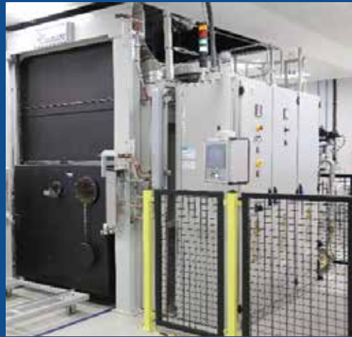
Industrial Oven: Working Dimensions: 1200 x 1200 x 1200mm Temperature: 400°C Vacuum Pump: 40 m 3 /h, 720 mmHg
