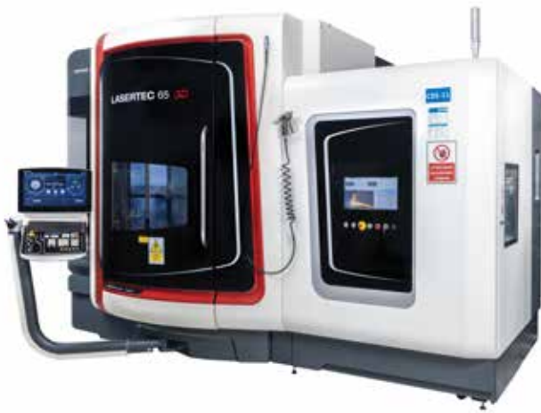
Direct Energy Deposition (Ded) Additive Method Building Volume: 650 x 650 x 560 mm Laser Power: 3000W
