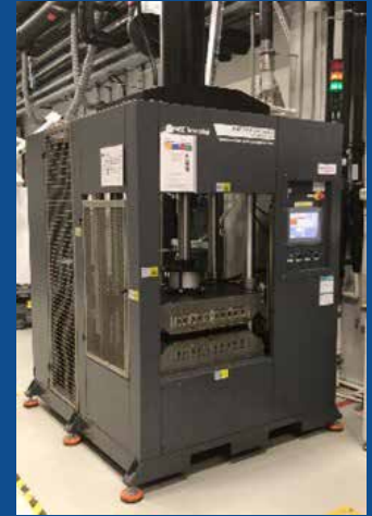
Dimensions : 500mm x 500mm Pressure Force: 50 tons Temperatura: 400°C
