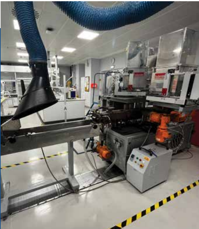
Twin Screw Extruder, Temperature Up to 350°C Throughput 25kg/h
