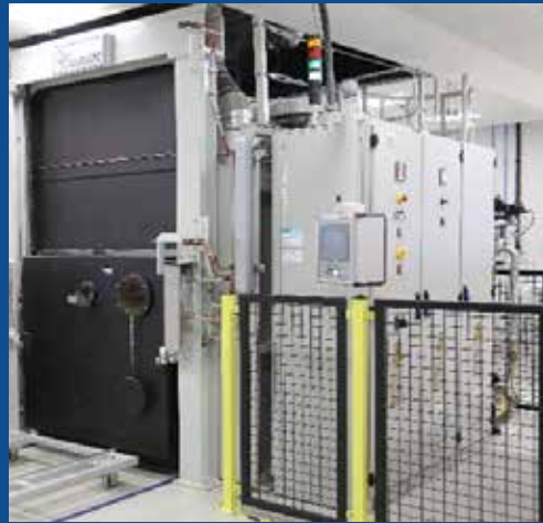
Working Dimensions: 1200 x 1200 x 1200mm Temperature : 400°C Vacuum Pump: 40 m 3 /h, 720 mmHg
