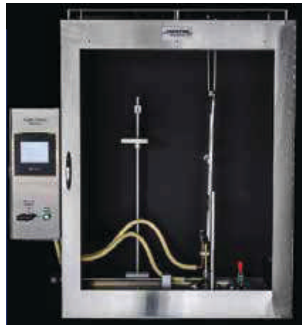
MULTIPURPOSE BURNER TESTER
