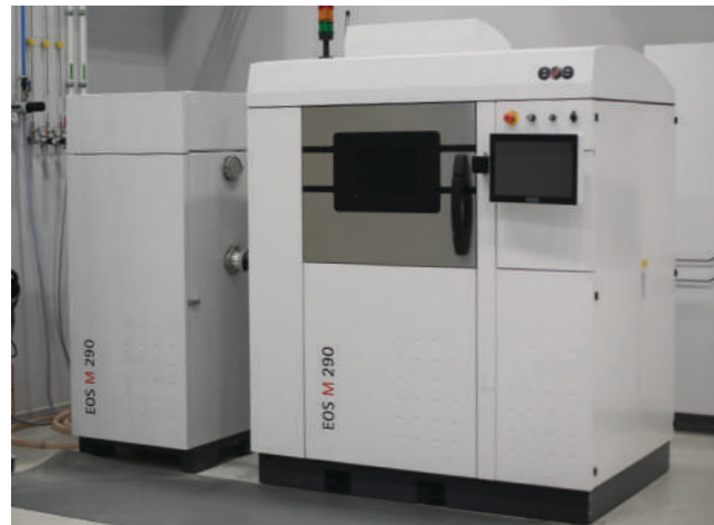
Selective Laser Melting Additive Method (SLM) Construction Volume: 250 x 250 x 325 mm Laser power: 400 W
